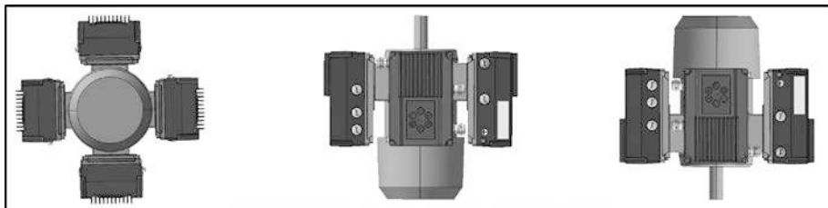
Fig.: 9 Motor installation location/permited alignments
