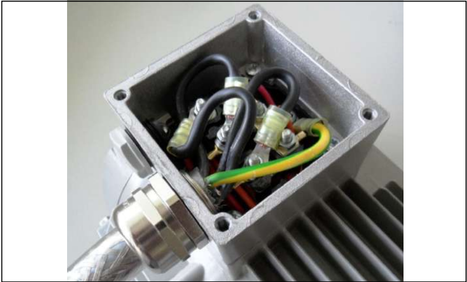
Fig.: 20 Wiring on the motor connection box
